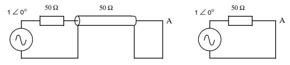
By inspection the voltage at point A is zero and the current is:  $\frac{1 \angle 0}{50} = 20 \angle 0$  mA.
