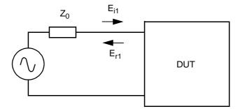
The voltage into the DUT is composed of 2 parts, an incident wave  $E_{i1}$  and a reflected one  $E_{r1}$  characterized by voltage and current :
